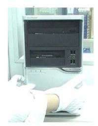
3. Rail the holder shown below, then take the ODD out from the chassis.
